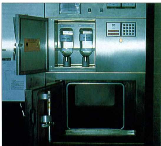
Figure 7 • Sterilizer showing the small canister of ethylene oxide attached to the door.
